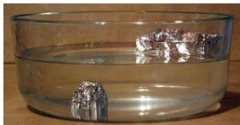
properly crushed aluminium foil sinks in water but it can float if it has trapped air
