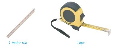
Fig. 1.5: Some common instruments to measure the length
