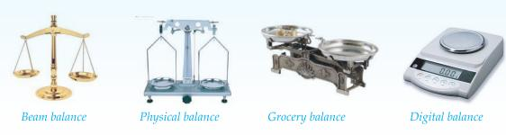
Figure 1.4: Some physical devices to measure mass
