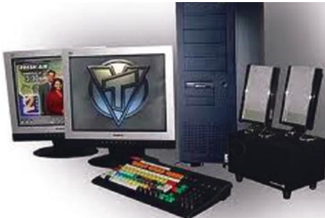
The NewTek Video Toaster was a combination of hardware and software for the editing and production of standard-definition video.
